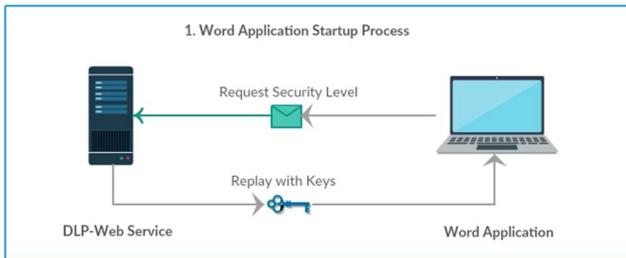
Figure 4. Word application startup process
