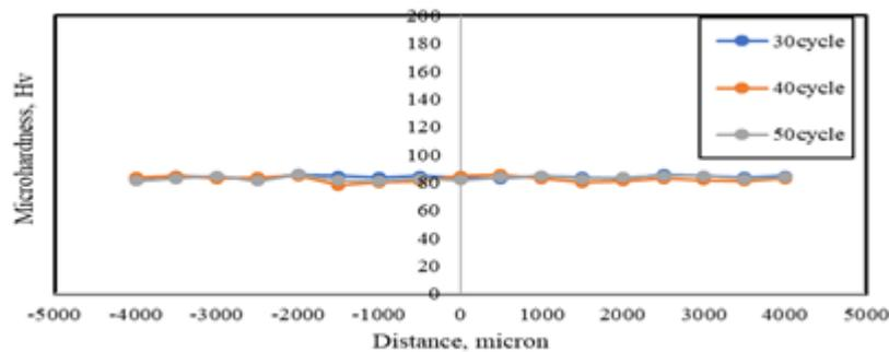
Figure 5. The hardness variation of the welding zone and matrix.
