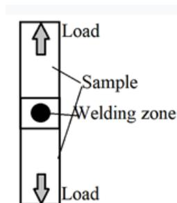
Figure 2. The tensile test geometry of the welding zone.
