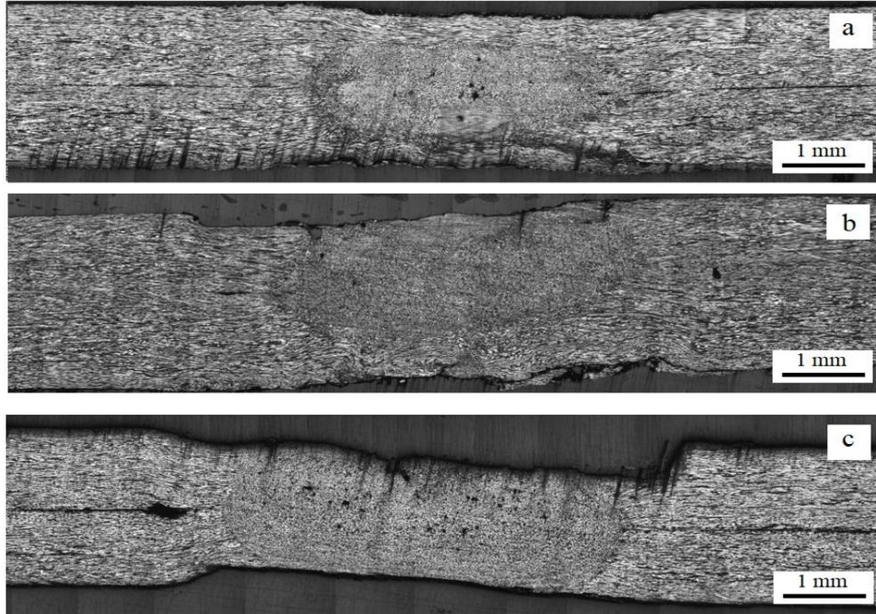
Figure 3. Optical micrographs of welded samples. a) 30 cycle b) 40 cycle c) 50 cycle
