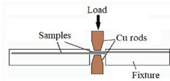
Figure 1. Resistance spot welding geometry.
