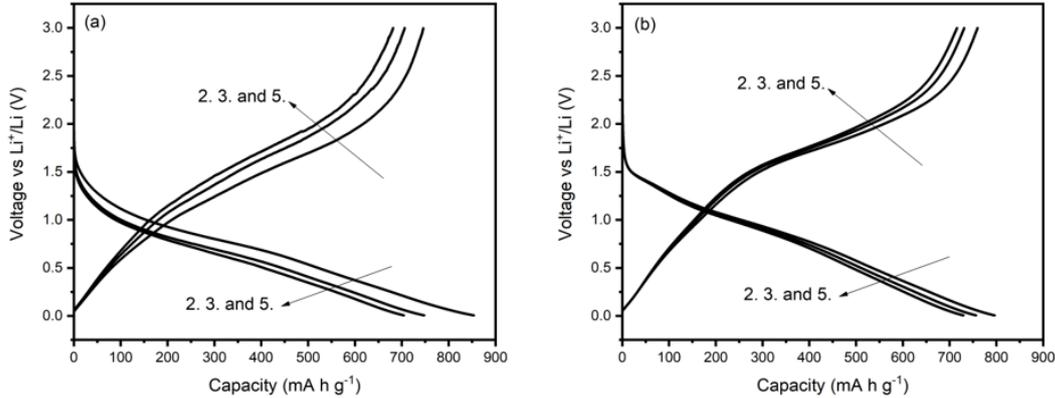
Figure 3. Discharge-charge curves of (a)  $\text{Co}_5(\text{MgNiZnLi})_{95}\text{O}$  and (b)  $\text{Co}_{35}(\text{MgNiZnLi})_{65}\text{O}$  anodes for the 2<sup>nd</sup>, 3<sup>rd</sup> and 5<sup>th</sup> cycles in the voltage range of 0.01-3.00 V at a current density of  $100 \text{ mA g}^{-1}$ .
