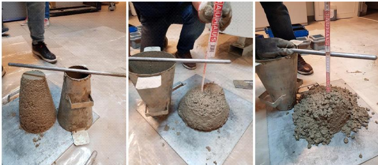
Figure 2. Measuring slump on mixtures B1(8), B2(16) and B3(31,5) (Beretin, 2020)
