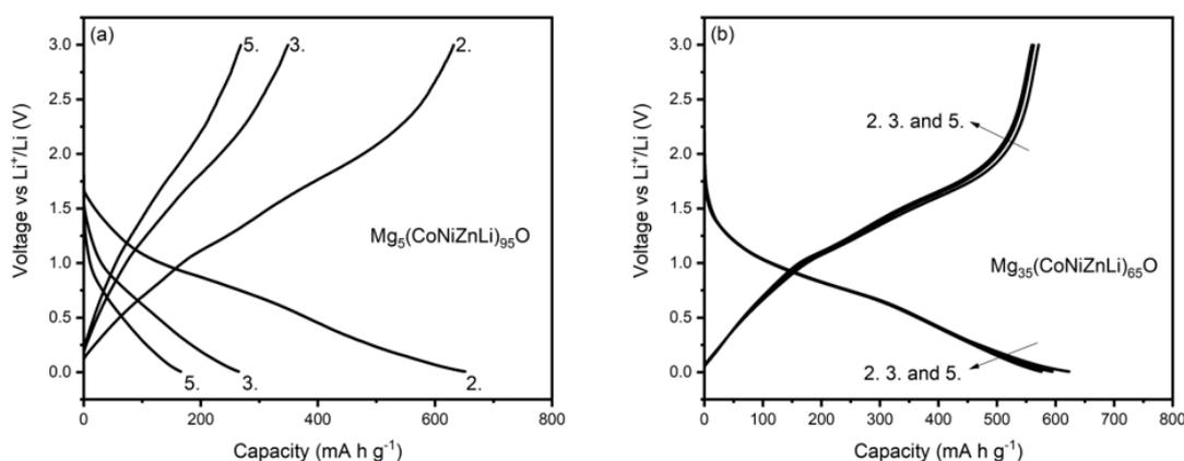
Figure 3. Discharge-charge curves of (a)  $\text{Mg}_5(\text{CoNiZnLi})_{95}\text{O}$  and (b)  $\text{Mg}_{35}(\text{CoNiZnLi})_{65}\text{O}$  anodes for the 2<sup>nd</sup>, 3<sup>rd</sup> and 5<sup>th</sup> cycles in the voltage range of 0.01-3.00 V at a current density of  $100 \text{ mA g}^{-1}$ .
