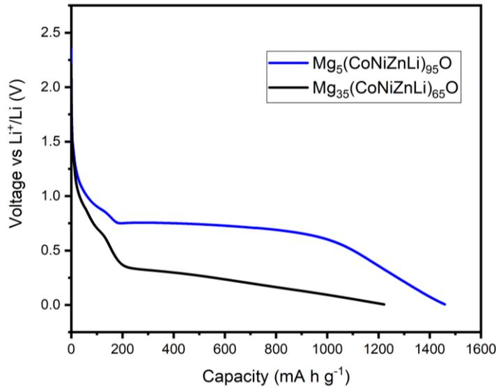
Figure 2. Initial discharge curves of Mg<sub>5</sub>(CoNiZnLi)<sub>95</sub>O and Mg<sub>35</sub>(CoNiZnLi)<sub>65</sub>O anodes at a current density of 100 mA g<sup>-1</sup>.
