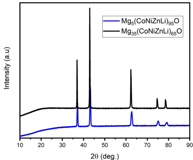
Figure 1. XRD patterns of the as-synthesized  $\text{Mg}_5(\text{CoNiZnLi})_{95}\text{O}$  and  $\text{Mg}_{35}(\text{CoNiZnLi})_{65}\text{O}$  HEOs.
