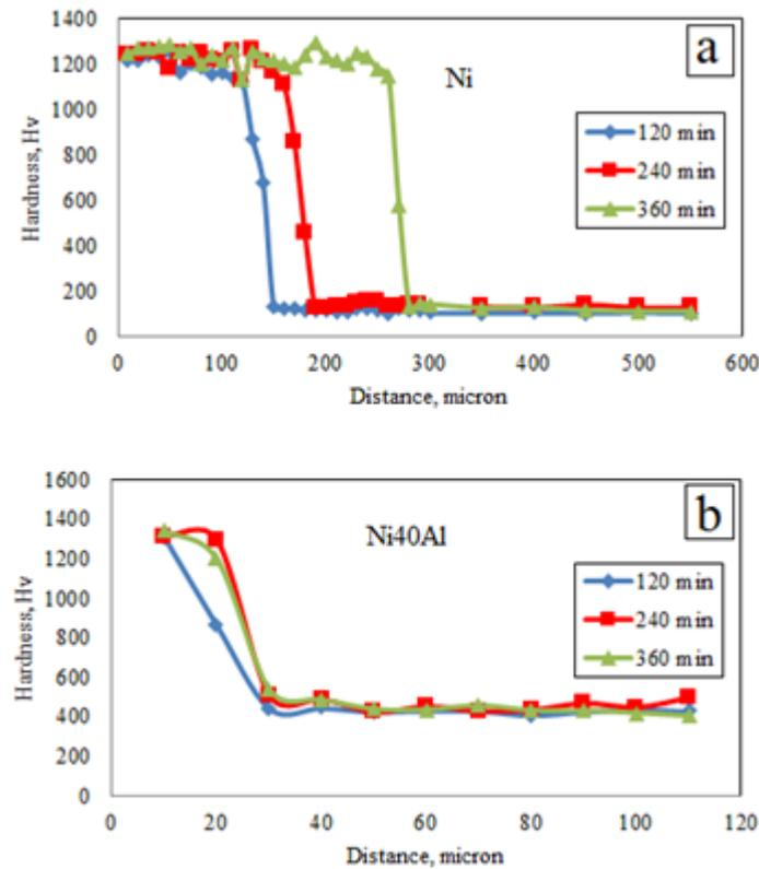
Figure 4. Microhardness values to the center from the borided samples. a) Ni b) Ni40Al
