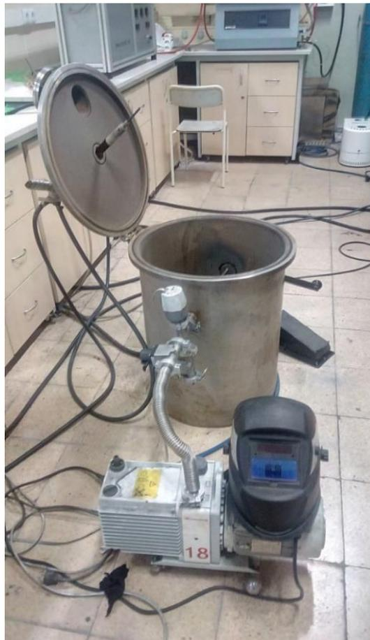
Figure 1. Vacuum arc melting furnace.
