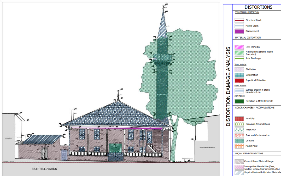
Figure 3. Layouts prepared in line with the detected deterioration and problems for Buğdaypazarı Mosque
