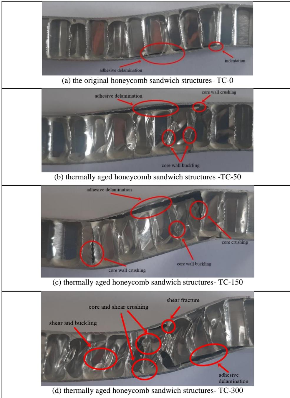
Figure 4. Failure modes of various thermally aged honeycomb sandwich structures after three-point bending tests
