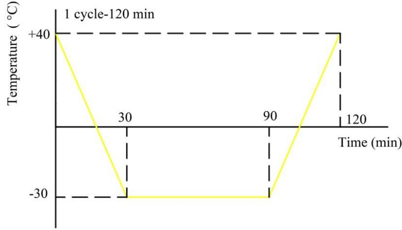
Figure 2. The temperature variations imposed during the accelerated thermal cycling test of honeycomb sandwich structures
