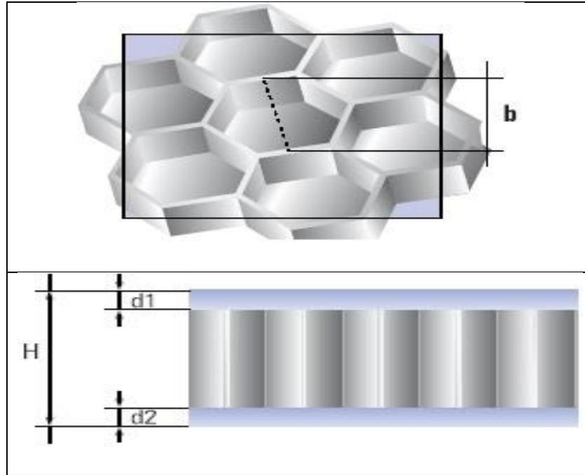
Figure 1. The geometry of honeycomb sandwich structures
