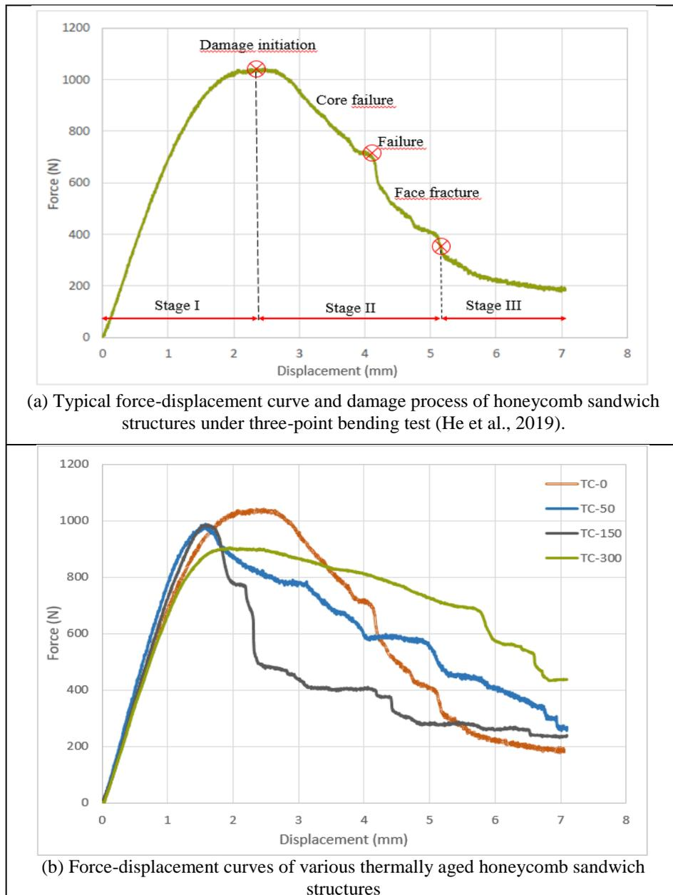
Figure 3. (a) Typical force-displacement curve and damage process of honeycomb sandwich structures under three-point bending test (He et al., 2019), (b) Load-displacement curves of various thermally aged honeycomb sandwich structures
