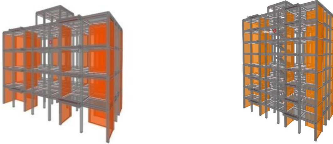
Figure 2. 3D FE models of the studied buildings made with CSi SAP2000 ver 15
