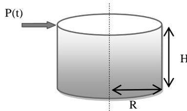
Figure 4. Tanks subjected to a concentrated load at the top.
