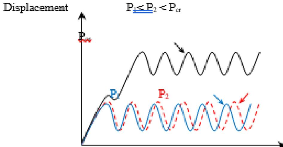
Figure 2. Detection of the critical load by criterion of Budiansky.
