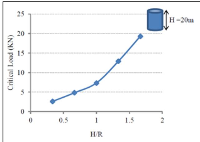
Figure 6. Variation of critical load versus h/r of tank h=20 m.
