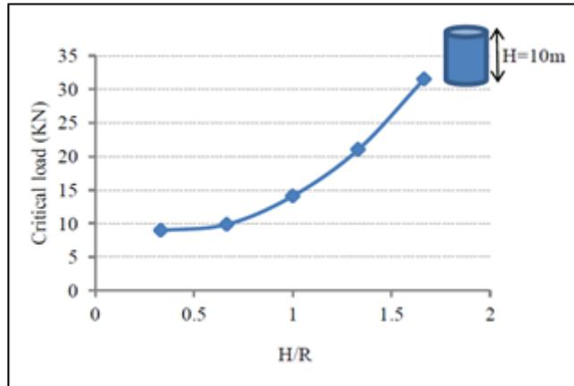
Figure 5. Variation of critical load versus h/r of tank h=10 m.
