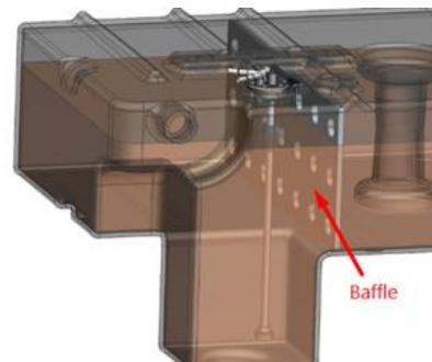
Figure 7: Breakwater Mechanism
