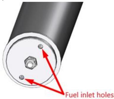
Figure 9: Placement of Fuel Inlet Holes on the Part
