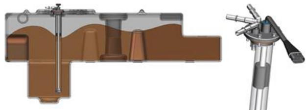
Figure 8: The Structure of the Housing Part on the Tank
