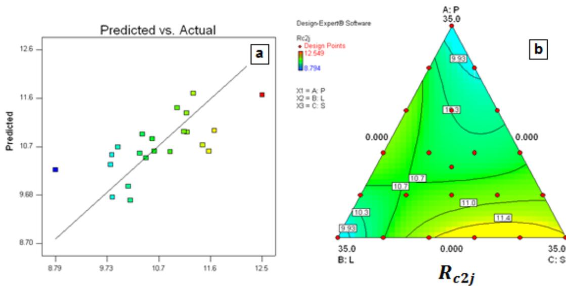
Figure 5. Compressive strength at 2 days a) Correlation between observed values and the model, b) Variation of compressive strength according to the model.
