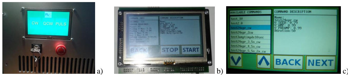
Figure 20. Laser work programming - a) laser working regime selection, b) example of QCW program, c) laser working regime example
