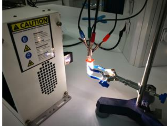
Figure 3. The photo-current measurements of CVD graphene - g-C 3 N 4 composites.
