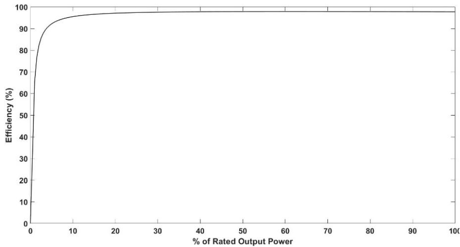
Figure 3: Typical efficiency curve for an inverter.
