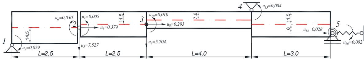
Figure 5. Displacements and rotations in the nodes
