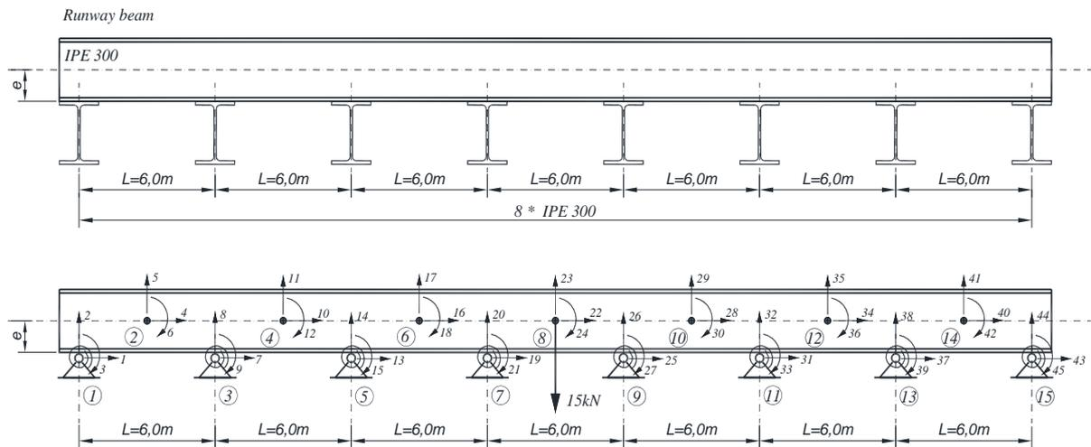
Figure 9. Crane beam
