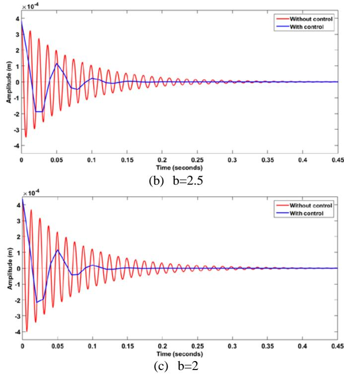
Figure 1. Impulse response of the smart beam for  $k=1$  (Actuators in FE2)
