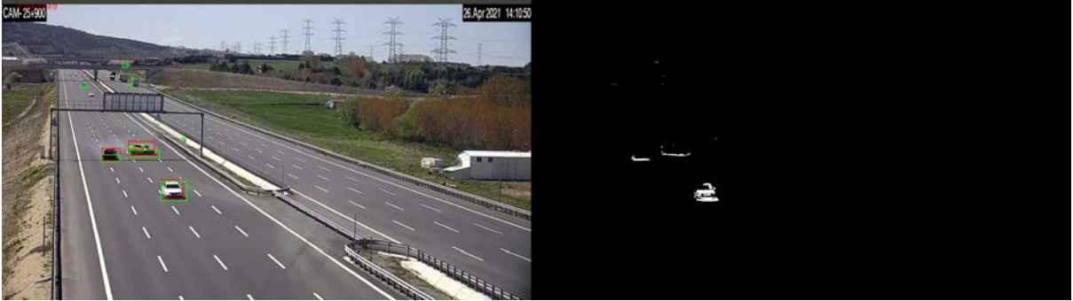
Figure 3. Sample motion mask and detected motion regions
