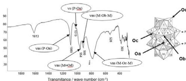
Figure 3. FT-IR spectrum of K<sub>6</sub>P<sub>2</sub>W<sub>12</sub>Mo<sub>6</sub>O<sub>62</sub>
