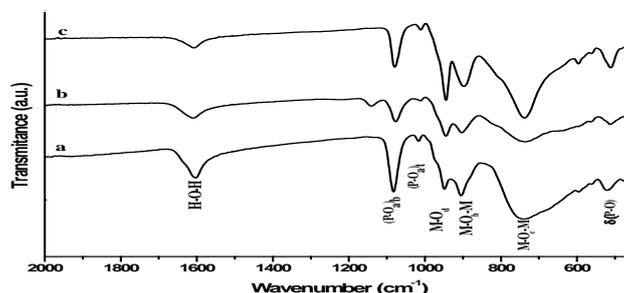
Figure 2. FT-IR spectra of (a) P<sub>2</sub>W<sub>12</sub>Mo<sub>6</sub>, (b) P<sub>2</sub>W<sub>12</sub>Mo<sub>5</sub>Sn (c) and CsSnP<sub>2</sub>W<sub>12</sub>Mo<sub>6</sub>
