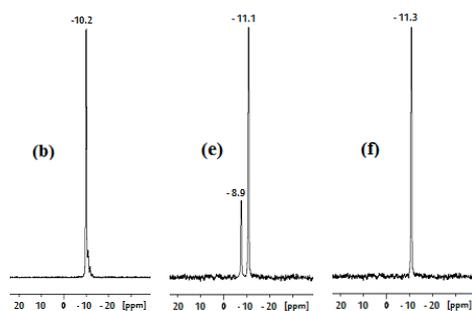
Figure 4.  $^{31}\text{P}$  NMR spectra of  $\alpha\text{-P}_2\text{W}_{12}\text{Mo}_6$  (b),  $\text{K}_7\text{P}_2\text{W}_{12}\text{Mo}_5\text{Sn}$  (e) and  $\text{Cs}_4\text{SnP}_2\text{W}_{12}\text{Mo}_6$  (f)
