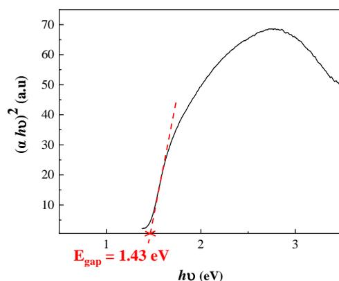
Figure 7:Tauc's plot for direct electronic transition
