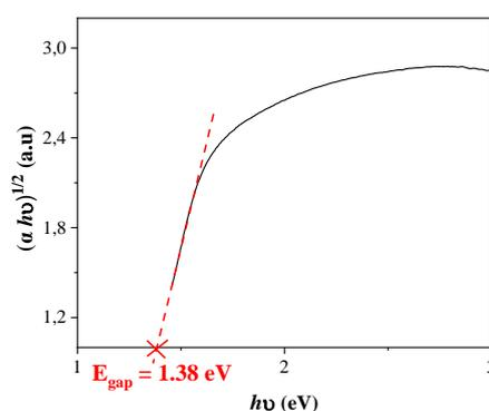
Figure 8. Tauc's plot for indirect electronic transition
