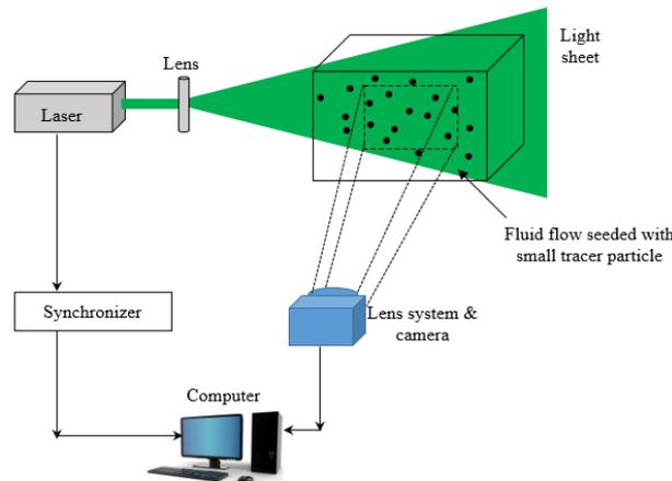
Figure 3. Schematic diagram of a PIV setup
