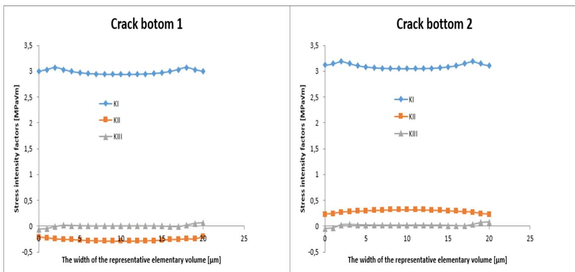
Figure 5. Variation of the stress intensity factors  $K_I$ ,  $K_{II}$  and  $K_{III}$  as a function of the width of the representative elementary volume alpha/epoxy for the two crack bottoms and for  $d_a=0\mu\text{m}$  and  $d_b=0\mu\text{m}$
