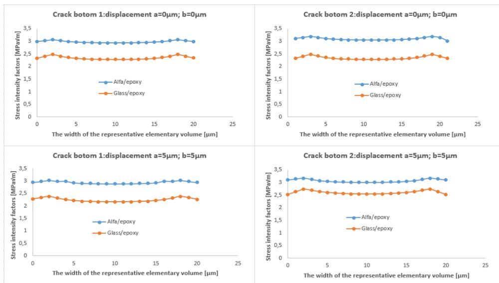
Figure 7. Variation of the stress intensity factor  $K_I$  as a function of the width of the representative elementary volume alfa/epoxy and glass/epoxy for the two crack tips and for  $d_a=0\mu\text{m}$  and  $d_b=0\mu\text{m}$  and  $d_a=5\mu\text{m}$  and  $d_b=5\mu\text{m}$ .
