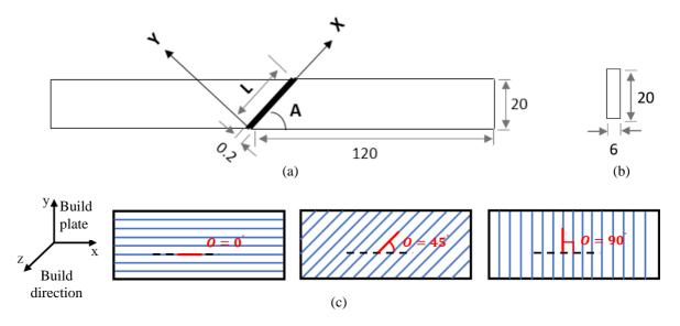
Fig. 1. Scarf joint specimen configurations (a) Top view of general configuration (b) Cross-sectional dimensions, (c) Three raster orientations of 0°, 45°, and 90° in 3D printing (from left to right, respectively). The build plate is on the xy-plane and the specimens are printed in z-direction.
