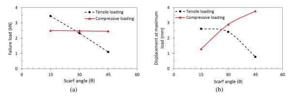
Fig. 9. Optimal design for scarf joints including adherends printed with a raster orientation of 45° attached by Araldite 2011. Optimization based on (a) failure load of the joints, (b) displacement at the maximum experienced load by the joints, as a function of scarf angle.
