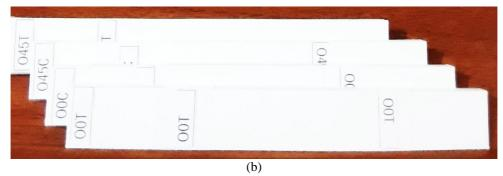
Fig. 2. Fabricated specimens (a) 3D printed PLA adherends in different scarf angles (A) and raster orientation (O), (b) the 3D printed single PLA specimens.
