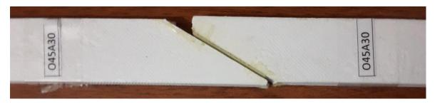
Fig. 10. Demonstration of the test specimens with the optimized scarf angle of 30°.
