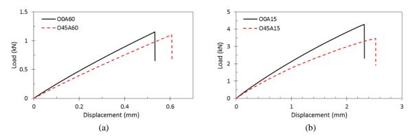
Fig.6 Comparison between the tensile behaviors of the joints including adherends of different raster orientations (i.e. 0° and 45°), (a) for the scarf angle of 60° (b) for the scarf angle of 15°.
