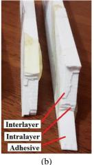
Fig.8 Debonding surfaces of two selected joints, (a) O0A60, and (b) O45A15. Different types of failure including Adhesive and Adherend (Interlayer and Intralayer) were labeled in the figures.
