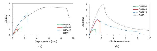
Fig.7 Comparison among the behaviors of the joints with different scarf angles (a) tensile test results (b) compressive test results. O45T and O45C show single adherends with a raster orientation of 45° under tensile and compression loadings, respectively. In the plot related to the compression tests (b), absolute values are given.
