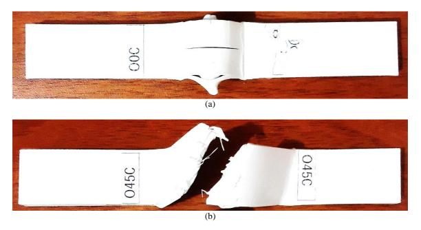
Fig.5 Failure images of single PLA specimens of different raster orientations in the compression test, (a) 0° raster orientation, (b) 45° raster orientation.
