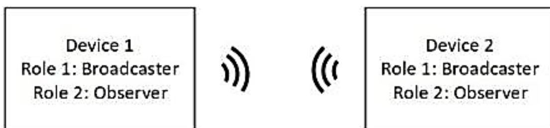
Figure 5. Overview proximity detection using BLE.
