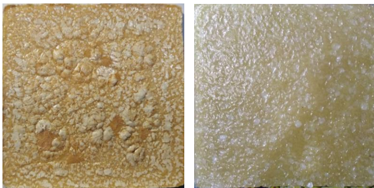
Figure 2. Photographs of the 40% lauric and paraffin composites
