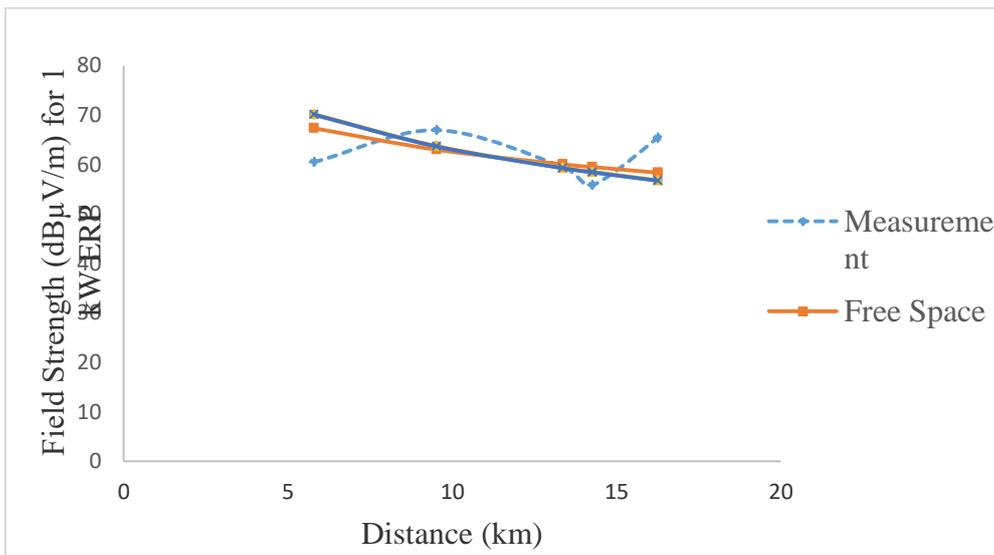
Figure 9. Modified field strength models for route C
