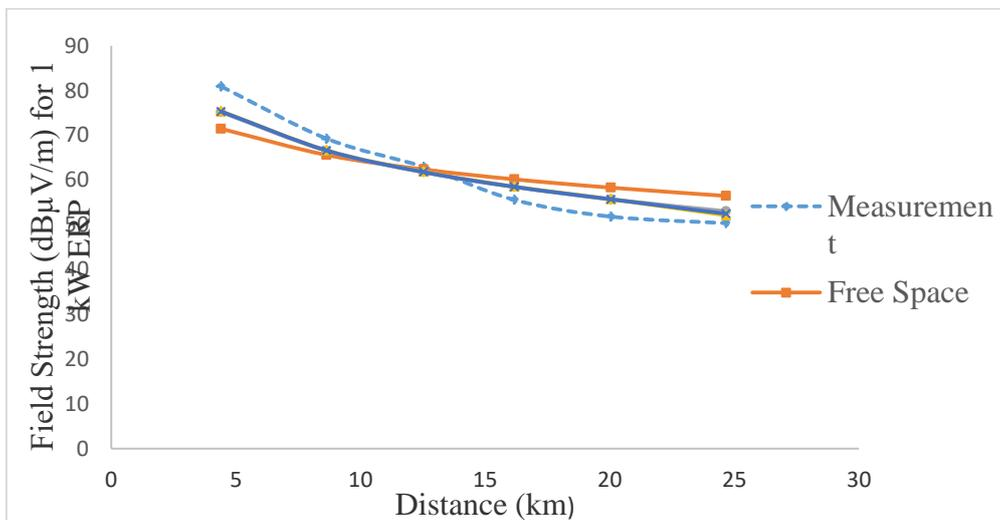
Figure 11. Generalised field strength models for route A
