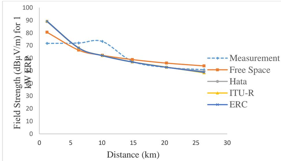
Figure 10. Modified field strength models for route D
