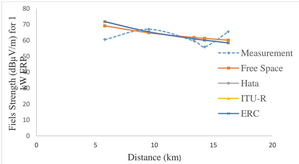
Figure 13. Generalised field strength models for route C
