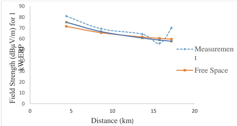
Figure 12. Generalised field strength models for route B
