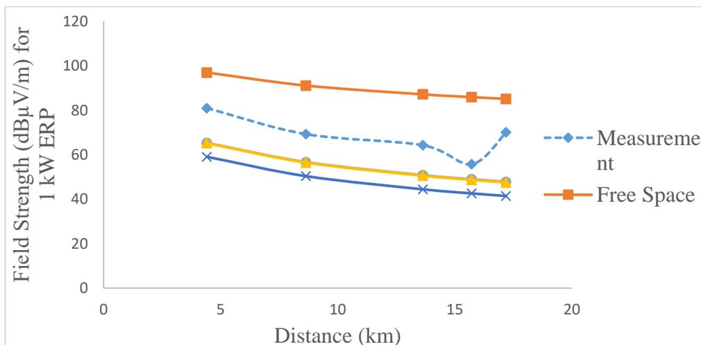
Figure 4. Field strength models for route B
