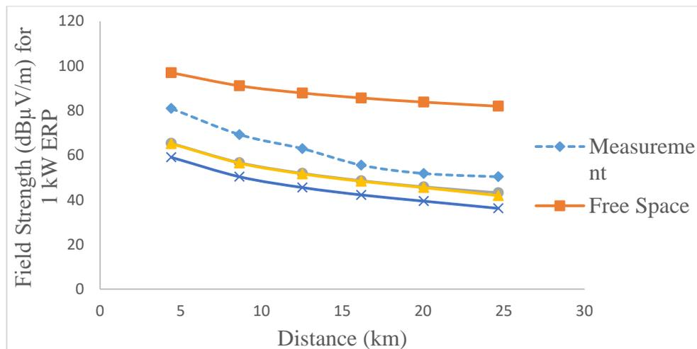
Figure 3. Field strength models for route A
