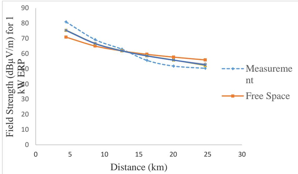
Figure 7. Modified field strength models for route A
