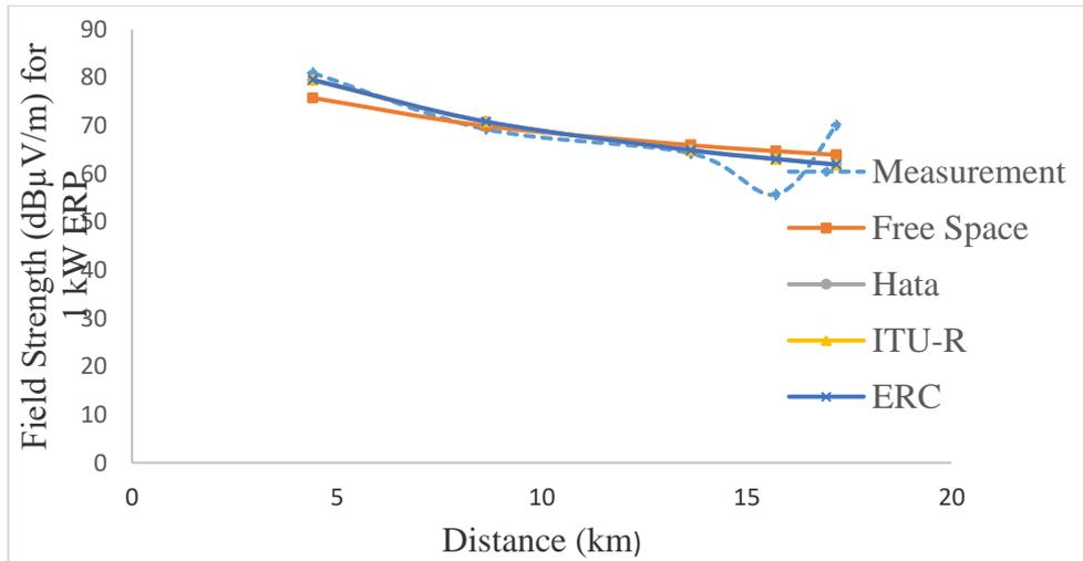
Figure 8. Modified field strength models for route B
