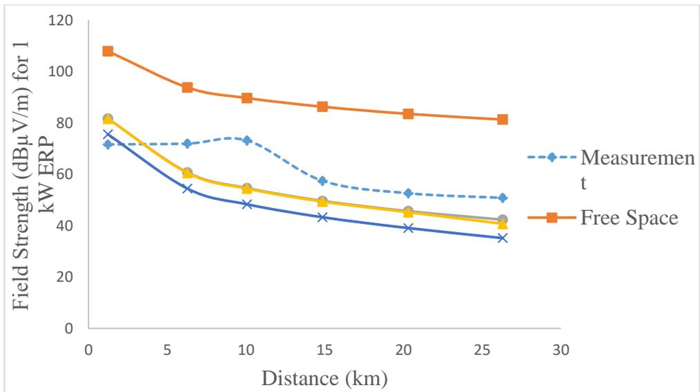
Figure 6. Field strength models for route D
