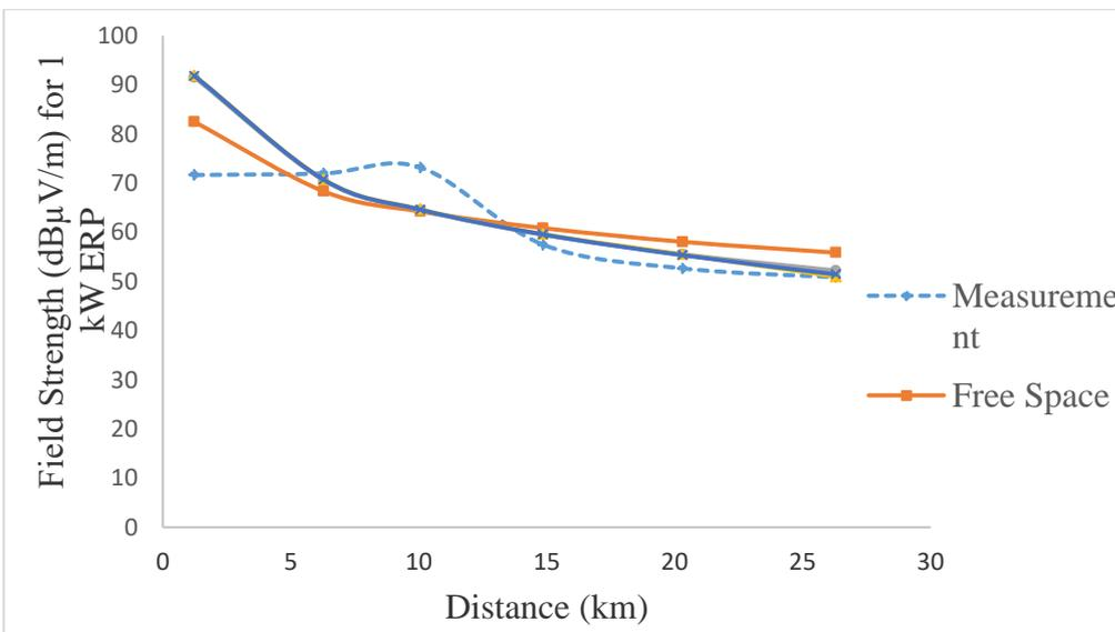
Figure 14. Generalised field strength models for route D
