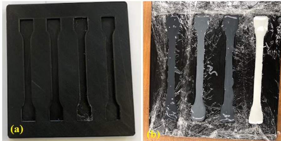
Figure 2. a) Mold prepared for bulk samples, b) bulk samples poured into the mold
