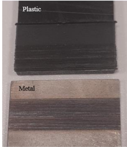
Figure 6. Image of broken parts from S7 specimen after tensile test.
