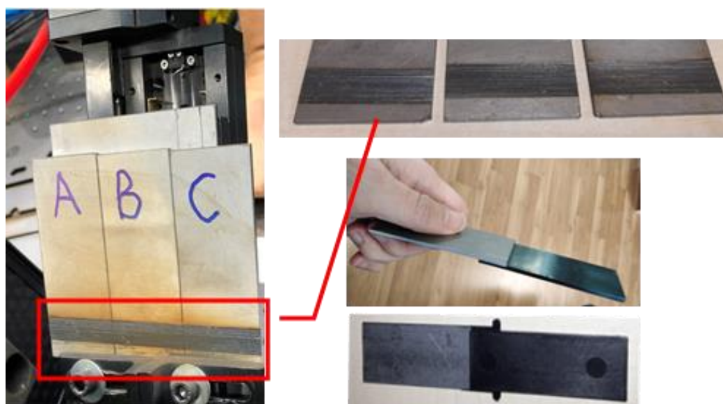
Figure 4. Surface-treated samples with channel structures and tensile test specimens (S6) and dimensions after plastic injection.
