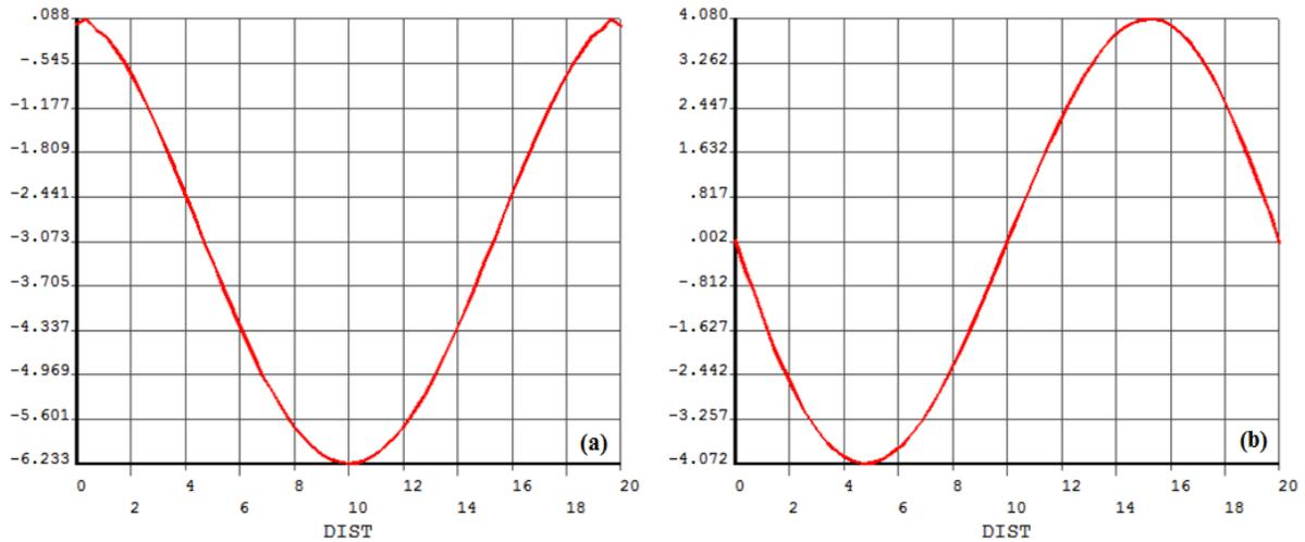
Figure 7. a) Normal stresses ( $\sigma_y$ ) and b) Shear stresses ( $\tau_{xy}$ ) distributions on the path
