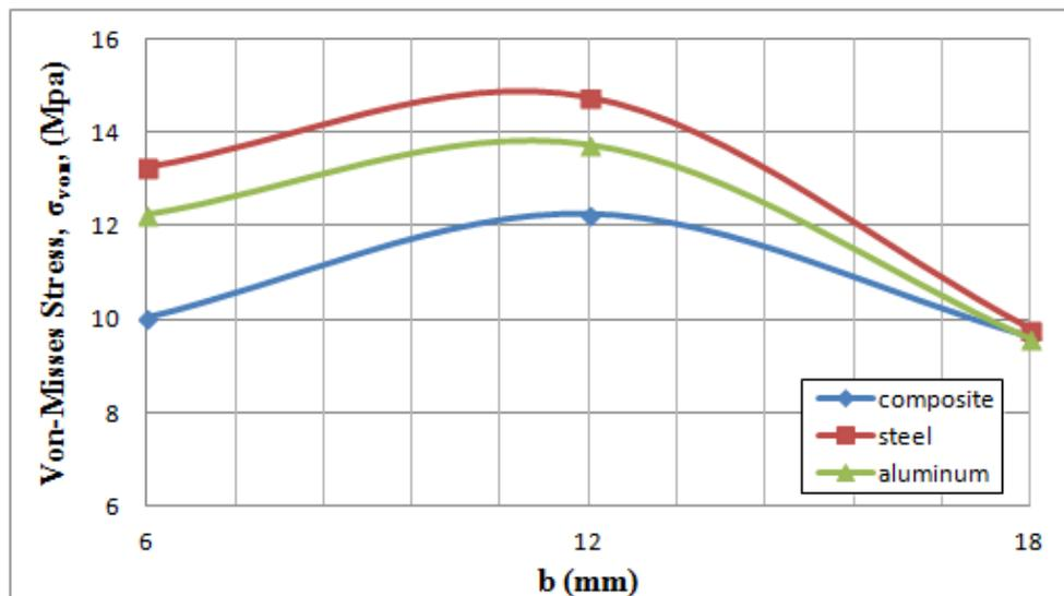
Figure 4. Von-Mises stress respect to diamond half length ( $b$ ) parameters.
