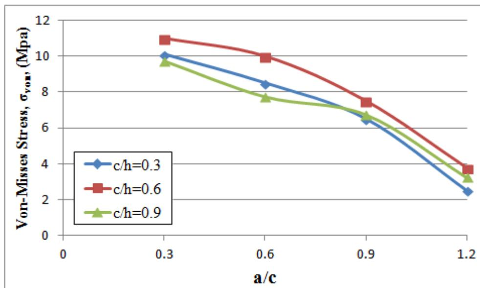
Figure 6. Von-Misses stress respect to a/c parameters
