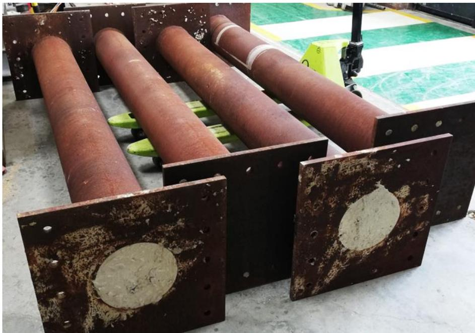
Figure 3. C5-C8 CFT specimens.
