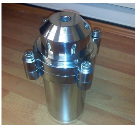
Figure 2. Photograph of designed and manufactured supercritical reactor.
