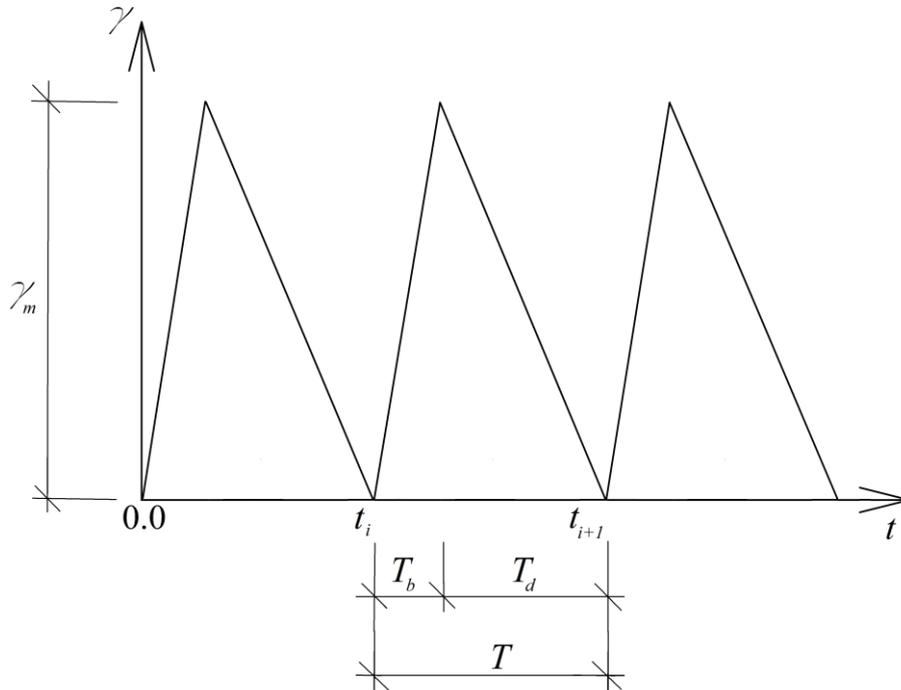
Figure 2. Periodic change of the shear strain.
