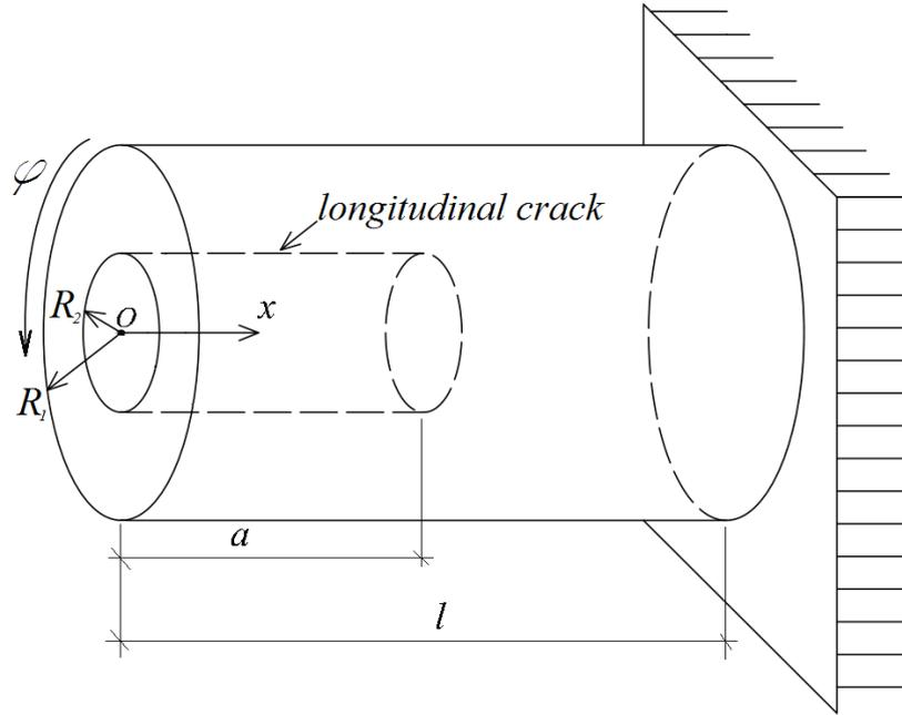
Figure 3. Static scheme of beam under examination.
