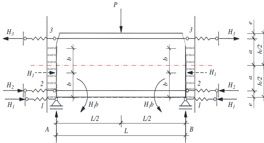
Figure 4. Supports of simple beam to columns
