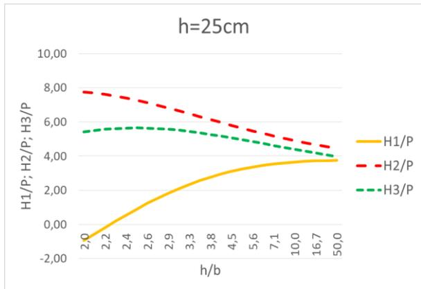
Figure 5. The parameters of the three support reactions - cantilever beam
