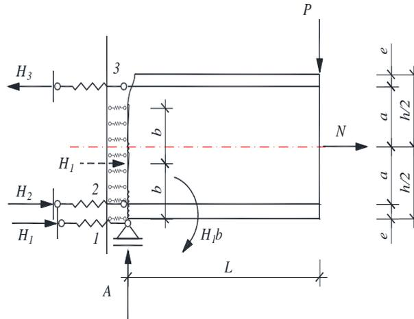
Figure 2. Supports of cantilever beam to column
