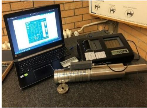
Figure 3. Surface roughness measurements with Mitutoyo SJ-310
