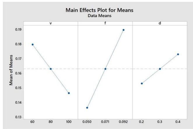
Figure 5. Main effects plot for Ra: a) for S/N ratio and b) for Means
