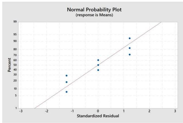
Figure 6. Normal probability charts for surface roughness
