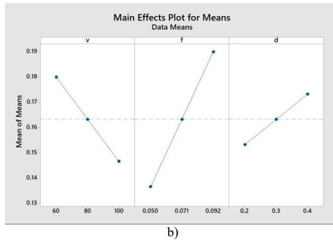
Figure 5. Main effects plot for Ra: a) for S/N ratio and b) for Means
