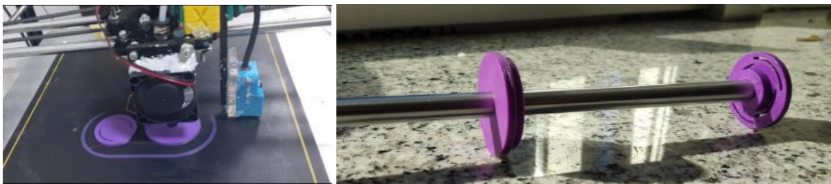
Figure 2. Shock absorber parts produced with 3D printer
