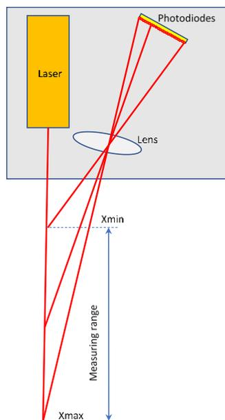
Figure 4. Triangulation principle.
