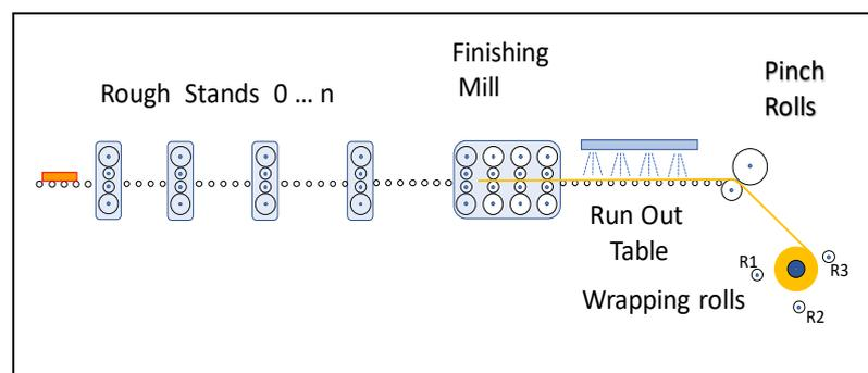
Figure 1. Hot strip mill layout.
