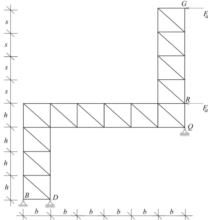
Figure 6. Statically indeterminate truss loaded by two forces.
