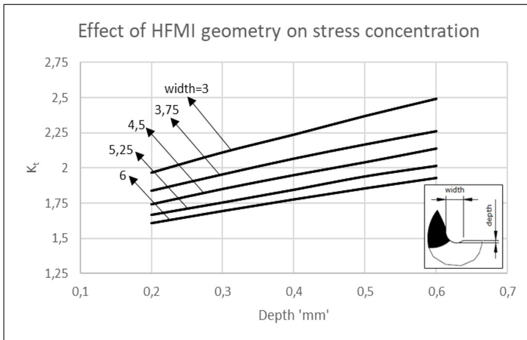
Figure 5. Effect of HFMI geometry on stress concentration
