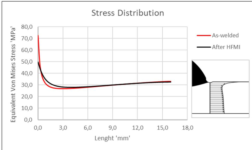
Figure 3. Stress distribution of as-welded and after HFMI
