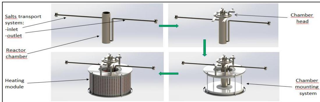
Figure 4. Reactor chamber design stages (made in SolidWorks)
