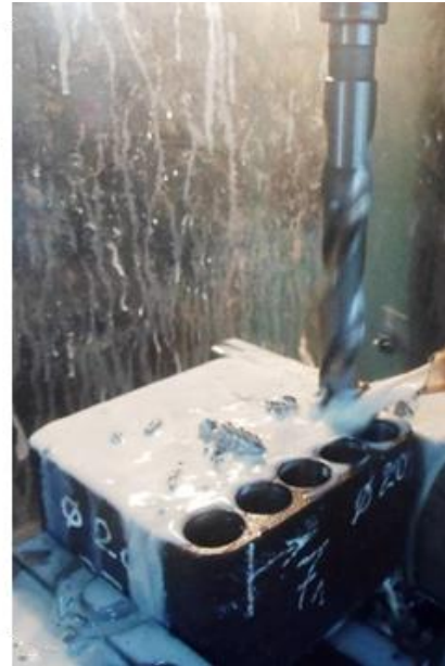
Figure 1. Specimen preparation hole repartition (25 holes for 20 mm diameter drill and 50 holes for 10 mm diameter drill) and photography of 20 mm hole blind drilling operation
