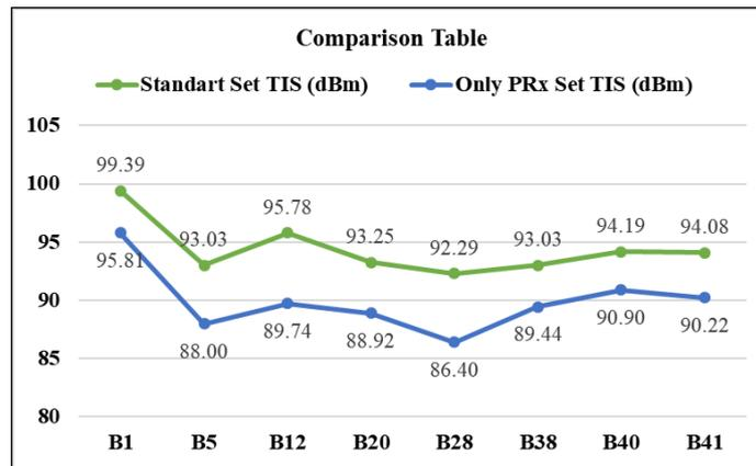
Figure 4. Comparison table for both FDD/TDD Bands
