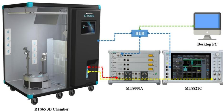
Figure 3. RTS65 3D chamber setup overview
