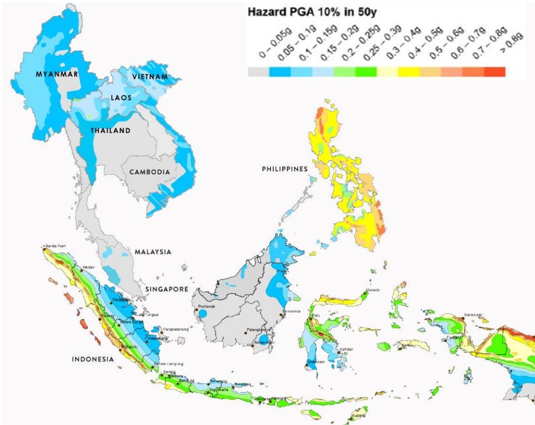
Figure 2. Final compilation of Southeast Asia seismic hazard map at 10% probability of exceedance in 50-year design period
