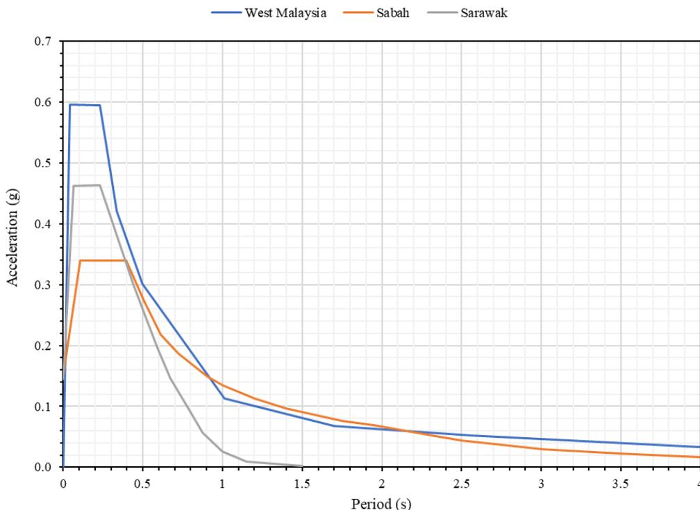
Figure 4. Design response spectra plotted at stable continental region by taking Malaysia as an example (the line shows three cities chosen for analysis (West Malaysia, Sabah and Sarawak))
