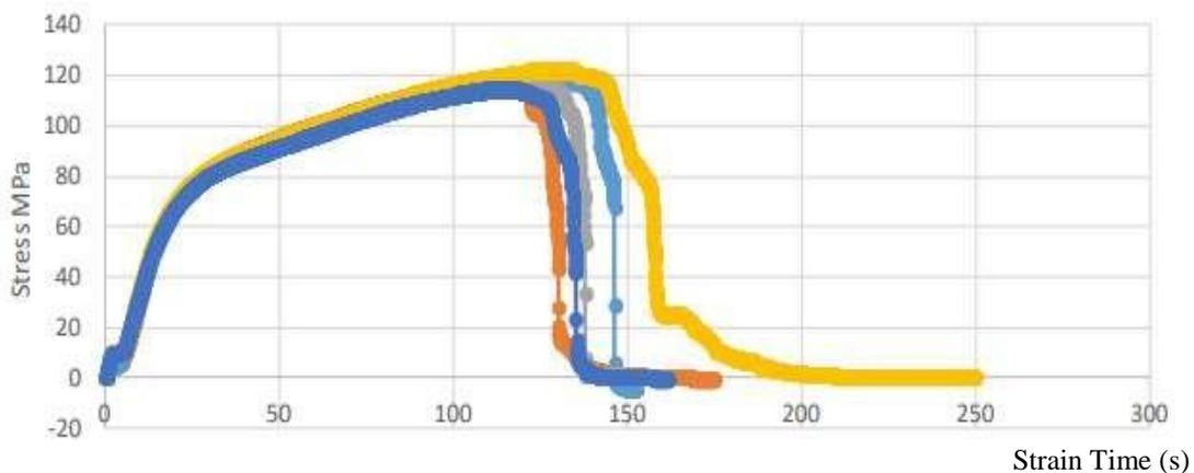
Figure 4. Stress vs. Strain times curves for CFRCs tested along  $45^\circ$  orientation.
