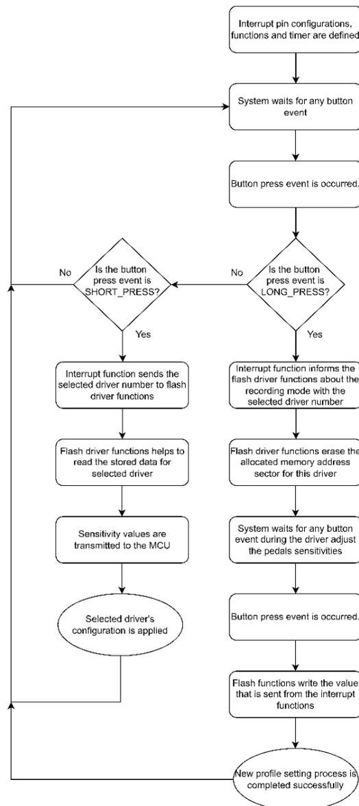
Figure 6. Flowchart for NVM management for different cases
