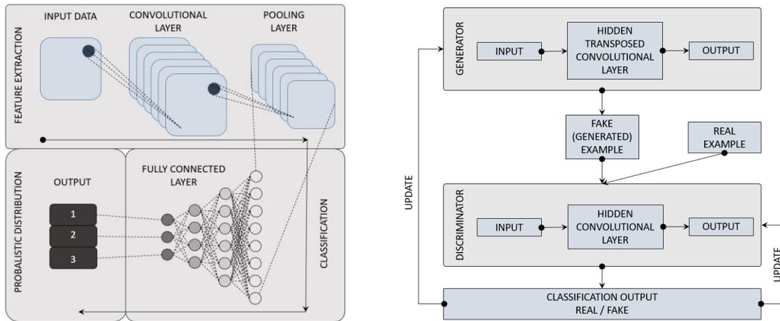
Figure 2. CNN architecture (left) and GANs workflow (right)
