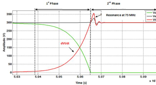
Figure 6. Voltages  $V_d$ ,  $V_e$ , and  $V_i$  during MOSFET transition to the locked state.
