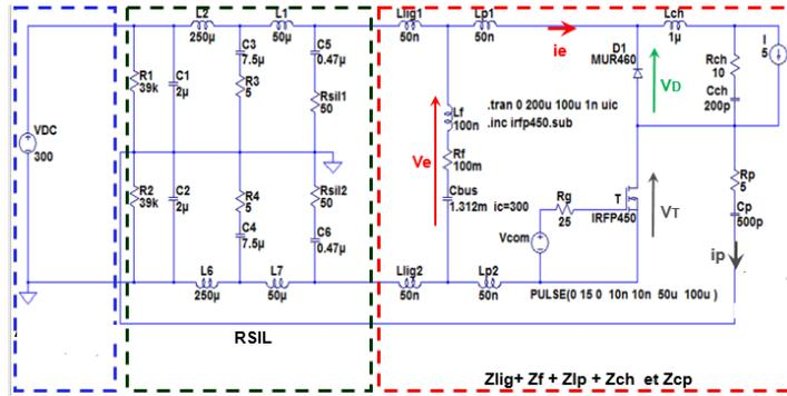
Figure 2. Simulation diagram of the series chopper supplied by a voltage source through the LISN.
