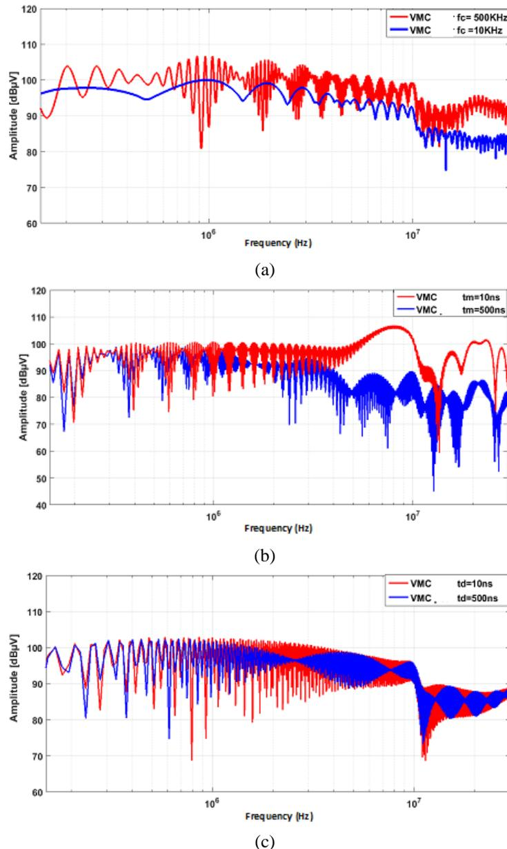
Figure 15. Influence of the switching frequency on the CM spectrum: (a)  $f_c$ , (b)  $t_m$ , (c),  $t_d$ .
