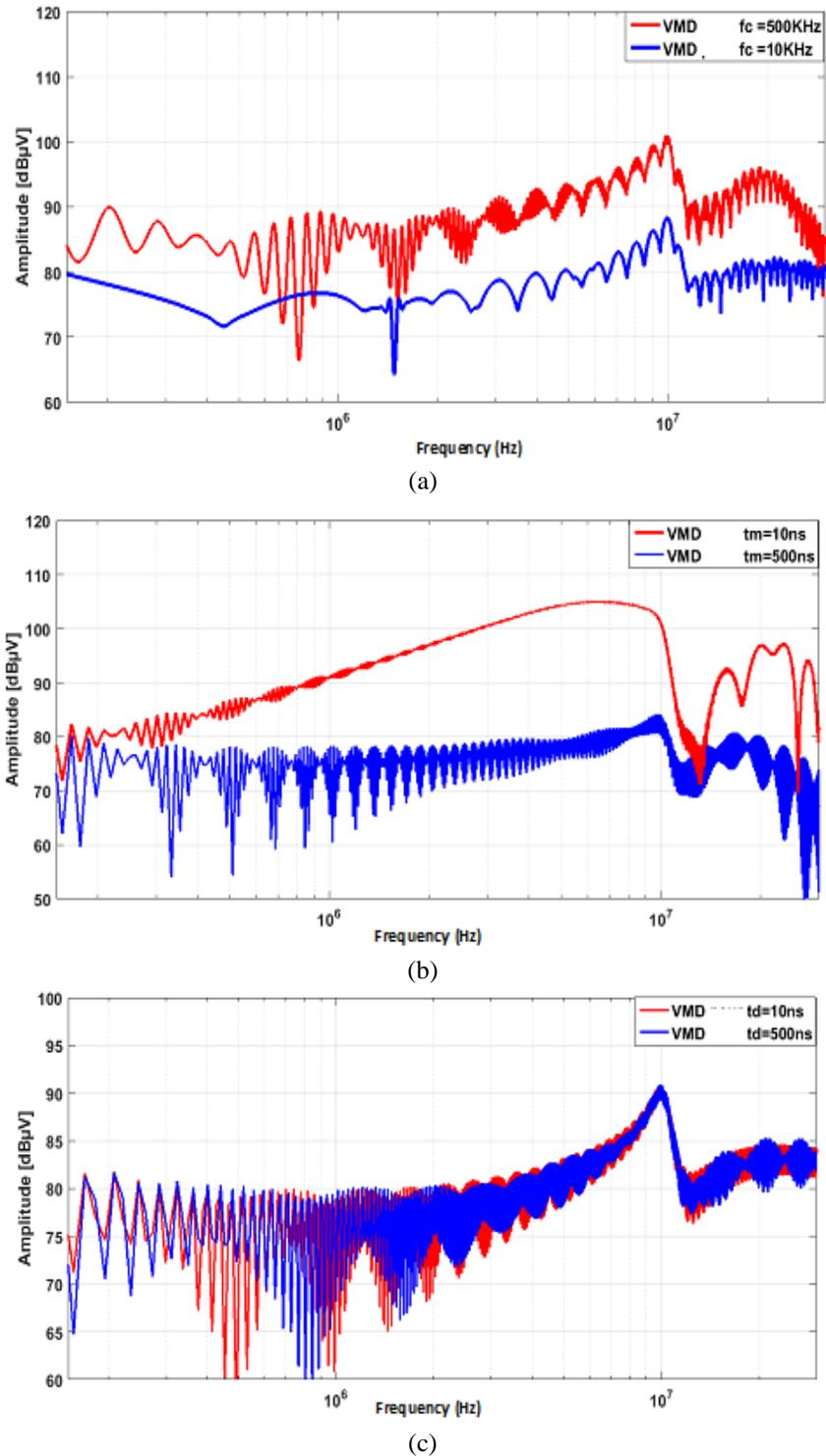
Figure 16. Influence of the switching frequency on the DM spectrum: (a)  $f_c$ , (b)  $t_m$ , (c)  $t_d$ .
