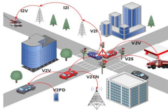
Figure 1. Communication between nodes in VANET network
