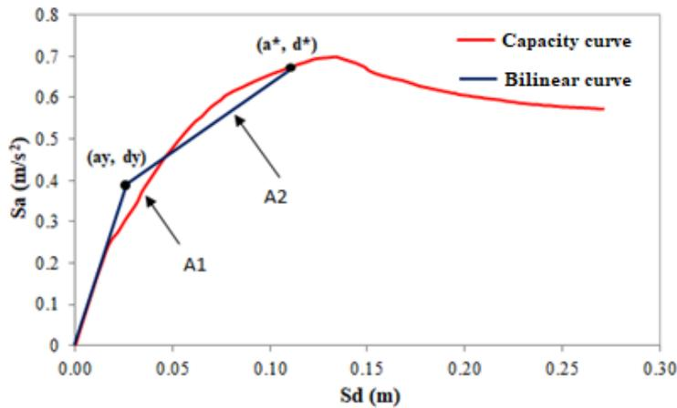
Figure 2. Capacity curve.
