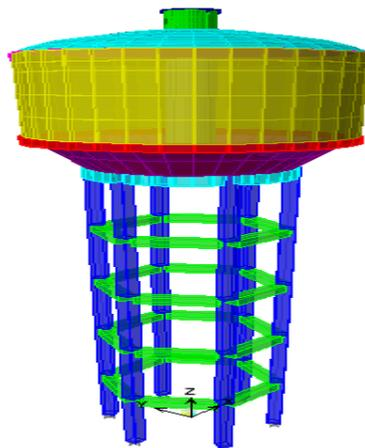
Figure 3. Finite element modeling of the elevated tank.
