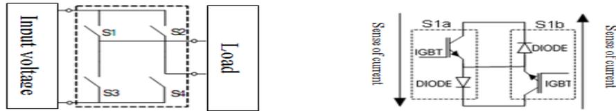
Figure 4. SPMC Structure, bidirectional switch module (Abrous, 2008)
