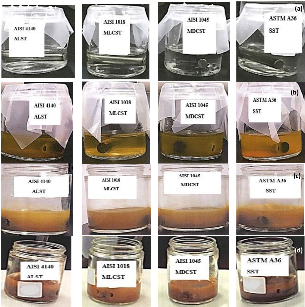
Figure 1. Photographs of steel alloys specimens during (a) week 1, (b) week 2, (c) week 5, and (d) week 8.
